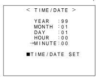
When the settings have been completed, press the SHIFT/ITEM button to select TIME/DATE SET and then press the UP (or DOWN) button. The time starts from when the button is pressed.
